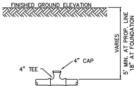
**TESTING TEE - ELEVATION**
